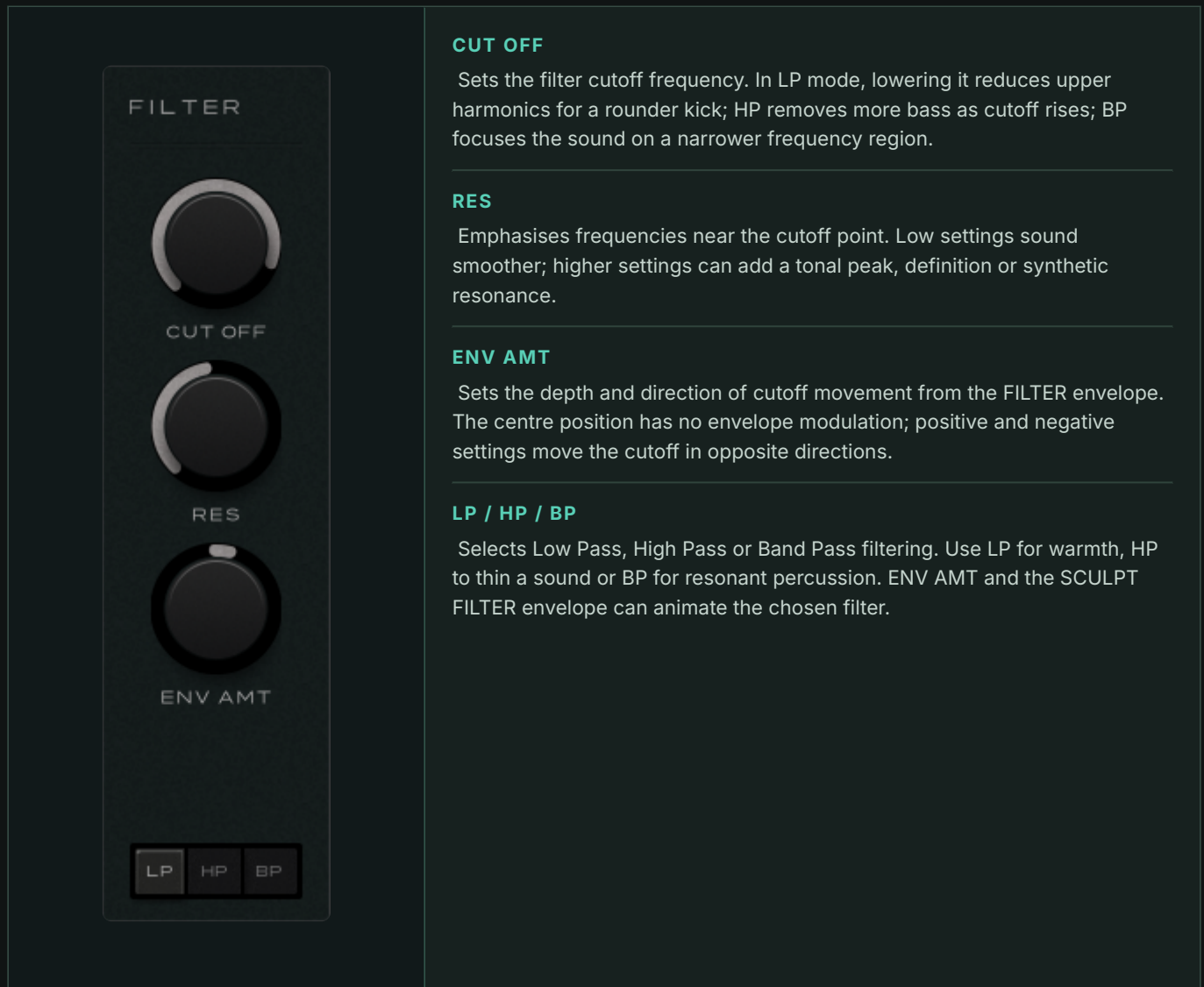
FIG 05 FILTER: cutoff, resonance, envelope amount and filter type.
